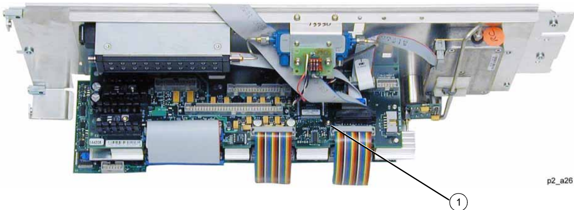
Figure 2-26 E8267D Microcircuit Interface Deck Top View
