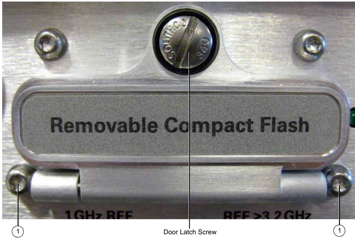
Figure 3-64 A41 Flash Drive Door Assembly
